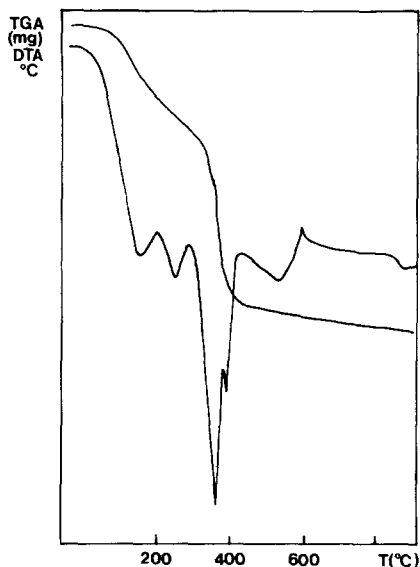
FIG. 7. Thermogram of MgO obtained at pH 3 (HCl).
